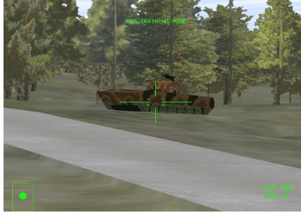
Figure 7. Unmanned Ground Vehicle (UGV) Gunner Sensor View. This is one of two 3D visualization screens the operator can use in controlling the UGV remotely.
